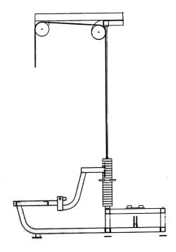
Figure 17. Lat pulldown cable routing.
